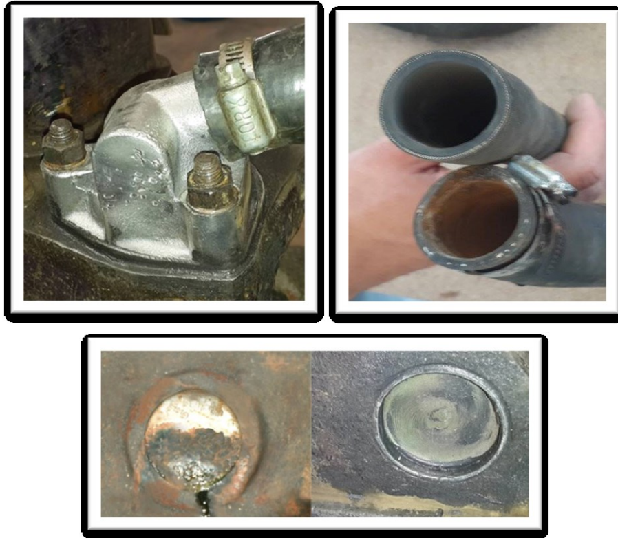
Figure 14 Rusted cooling system components compared with new parts
