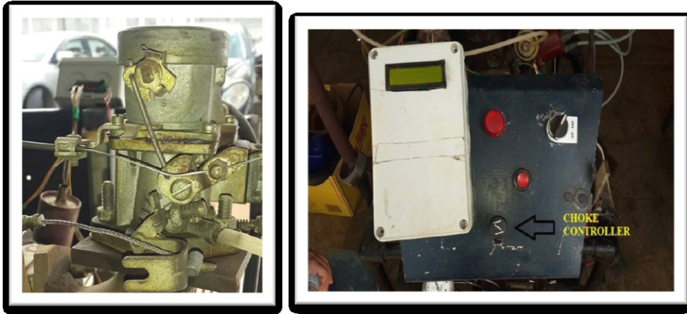
Figure 16 Installed choke and control unit display.
